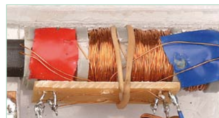
Figure 3. Inductors L1 and L2 are wound on a ferrite rod with a diameter of 10 mm and a length of 100 mm.
