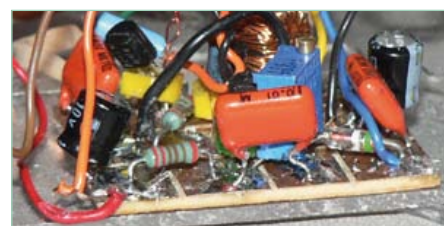
Figure 4. This close-up shows how to solder the components onto the board.
