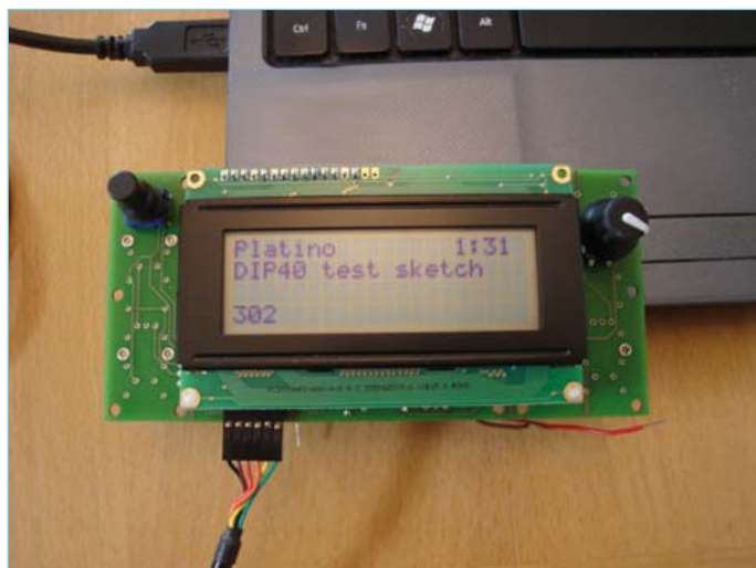
Figure 3. The test sketch from Figure 2 running on Platino. The value in the lower l/h corner (302) is controlled by the rotary encoder at the right; the timer in the upper r/h corner can be reset with the pushbutton on the left.
