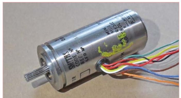
Figure 8. One of the motor/tachogenerators units.
