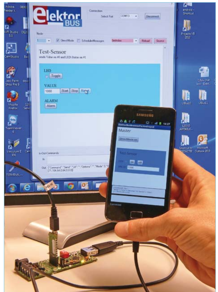
Figure 6. Initial testing can be performed by connecting the AndroPod to a PC (for example over the BOB FT232 USB to TTL converter).
